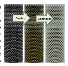
an inert carrier gas to ensure stable reaction conditions. Additively manufactured periodic open cellular structures (POCS) composed of Ti-6Al-4V (Ti64) alloy, with
