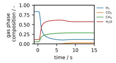
Figure 1: Simulated outlet composition of an isothermal PFR after an instantaneous change of the inlet composition. At time t = 0 s, a change of inlet composition was simulated from hydrogen excess (H2/CO2 = 19/1 mol/mol) to stoichiometric feed composition. Reaction conditions: T =  $300^{\circ}$ C, p = 10 bar, flowrate =  $0.5 \text{ ml}_{\text{STP}}$  min<sup>-1</sup> mg<sub>cat</sub><sup>-1</sup>. The underlying kinetic model is able to describe the dynamics of the catalyst.
